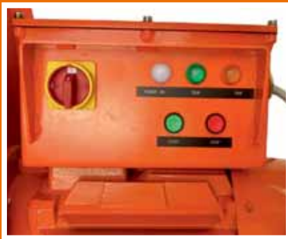
Die cast electrical box with main switch and overload relay.
